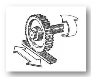
Velocity ratio (rotary to linear motion)
